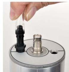
Attach air hose to one fitting
