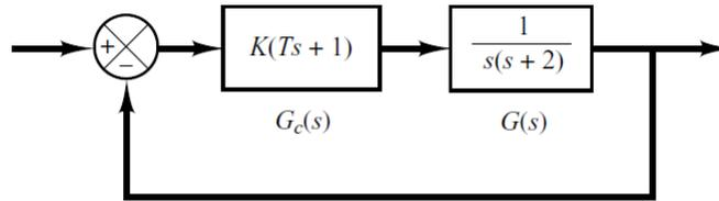
find  $K, T$  such that the desired closed loop system poles are located at  $-2 \pm j2$ . Plot the step response before and after the addition of the compensator to the system.
