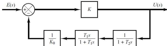
shows the block diagram representation of a compensator  $(U(s)/E(s))$ . Prove that this block diagram can be reduced into a PID controller with the three gains for the proportional, derivative, and integrator components. Derive these constants, i.e., derive  $K_i, T_i, T_d$  in terms of  $K_0, T_1, T_2, K$ .
