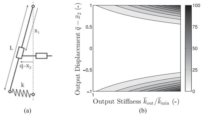
Fig. 6. VSAwVLA—(a) Schematic representation. (b) Squared input force  $\bar{f}_{in}^2$  over the workspace of this stiffness tuning mechanism.
