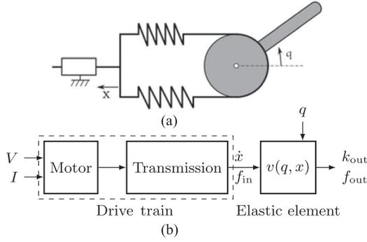
Fig. 1. Model of a variable stiffness mechanism. (a) Example of an antagonistic variable stiffness mechanism. (b) Schematic representation of the stiffness modulating subsystem, where  $V$  denotes the applied voltage to the motor,  $I$  denotes the motor current,  $\dot{x}$  is the velocity at the input to the mechanism,  $f_{in}$  is the force imposed by the mechanism to the drive-train,  $f_{out}$  is the output force, while  $k_{out}$  is the output stiffness of the actuator.
