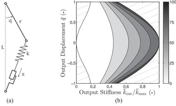
Fig. 3. MACCEPA—(a) Schematic representation of the stiffness adjusting subsystem. (b) Squared input force  $\bar{f}_{in}^2$  over the workspace of the mechanism. The dimensionless model parameter is  $\bar{r} = 1/5$ . The plot represents a typical behavior of this system.
