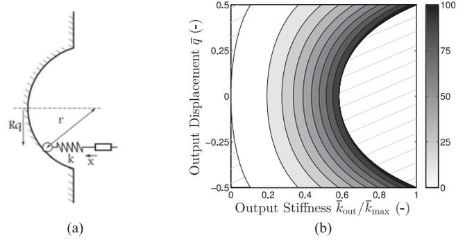
Fig. 4. VS-Joint—(a) Schematic representation of the stiffness modulating mechanism. (b) Squared input force  $\bar{f}_{in}^2$  over the workspace of the mechanism.
