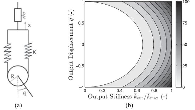
Fig. 2. Antagonistic variable stiffness mechanism. (a) Schematic representation of the reduced mechanism dedicated to stiffness modulation. (b) Squared input force  $f_{\text{in}}^2$  over the workspace of the mechanism. The black lines denote constant  $f_{\text{in}}^2$  curves. Darker colors denote higher values of the force.
