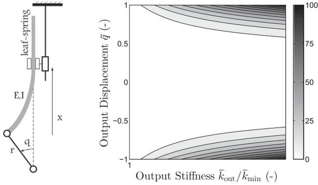
Fig. 7. VLLSM — (a) Schematic representation. (b) Squared input force  $\bar{f}_{in}^2$  over the workspace of this mechanism.
