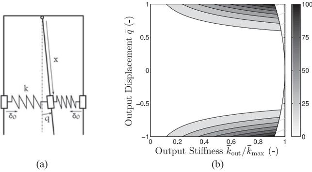
Fig. 5. AwAS—(a) Schematic representation of the stiffness adjusting mechanism. (b) Squared input force  $\bar{f}_{in}^2$  over the workspace of this stiffness tuning mechanism.
