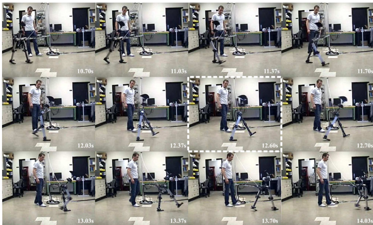
Fig. 9. Actuated dynamic walking—frame sequence extracted from the experimental video. The motion frame marked with dashed white line depicts the preemptive ankle push phase when only the toe on the rear foot is on the ground.
