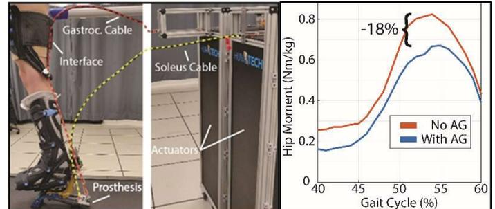
**Figure 1:** Experimental Set-up (left), Example of Prosthetic Side Hip Torque with vs. without the AG (right).
