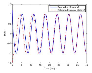
**Fig. 2.** The simulation for state  $x_2$  by the full-order observer (5).
