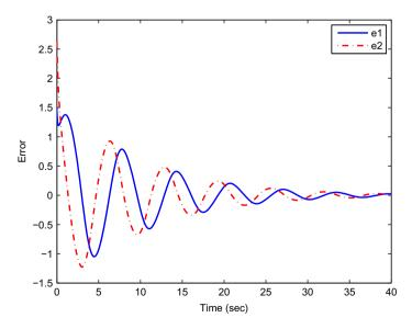
Fig. 3. The simulation for the error dynamics of the full-order observer (5).
