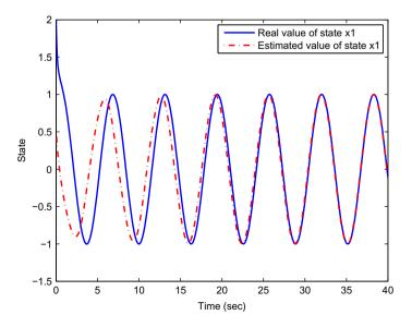
**Fig. 1.** The simulation for state  $x_1$  by the full-order observer (5).
