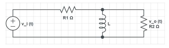
(a) (10 points) Derive the transfer function  $\frac{V_o(s)}{V_i(s)}$  in terms of  $R_1$ , L, and  $R_2$ . Show your work.
