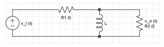
(a) (15 points) Derive the transfer function  $\frac{V_o(s)}{V_i(s)}$  in terms of  $R_1$ , L, and  $R_2$ . Show your work. Your transfer function should have the standard form of a transfer function, i.e., polynomials in the numerator and denominator.
