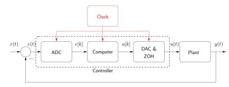
What is zero order hold? It's basically the model of the signal reconstruction of the digital to analog converter (DAC):
