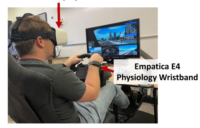
Virtual-Reality Driving Simulator with Artificial **Intelligence-based Analysis and Feedback**
