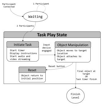
Fig. 4. Generic finite state machines for all tasks
