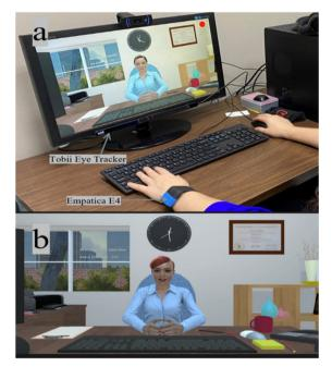
**Fig. 1.** CIRVR job interview simulator: (a) desktop-based interaction setup with Tobii eye tracker and the Empatica E4 physiological-sensing wristband; (b) desktop-based interaction view of the interviewer
