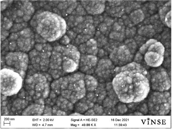
**Figure S2** I SEM of electropolymerized PPy grown on gold at a potential of 1 V for 30 s with  $NaClO_4$  as a dopant.
