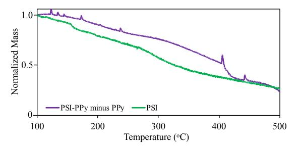
**Figure S5** Normalized TGA comparing the relative mass loss of PSI in both the pure and PSI-PPy samples.
