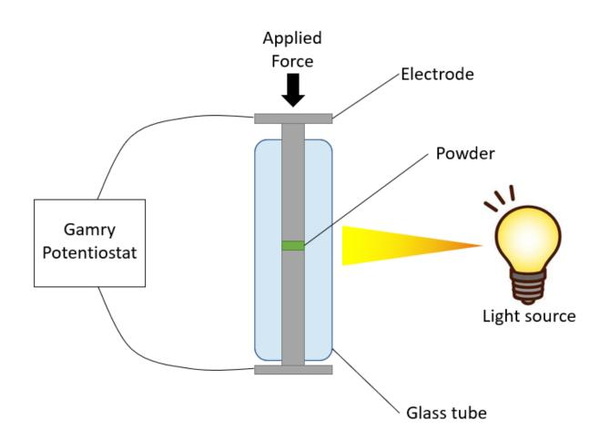
**Figure S7 I** *Two-piston experimental setup to measure conductivity and photoresponse for powder products.*
