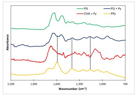
Figure S1 | Infrared spectra of films prepared from PSI (top), electropolymerized Ppy (bottom), as well as separate spectra for PSI and chlorophyll a that were exposed to Py and NaClO<sub>4</sub> under irradiation with a solar simulator for 6 h. The dashed lines indicate the position of prominent peaks in the Ppy control spectrum.
