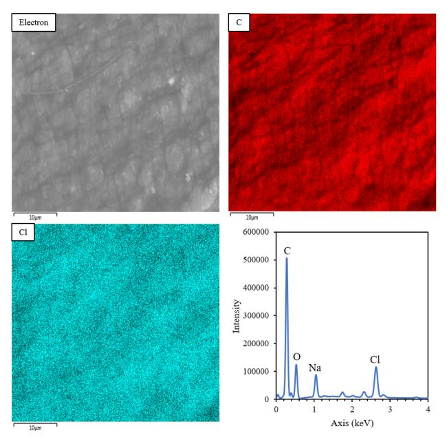
**Figure S3** | *EDS map and spectra of PSI-PPy powder showing presence of Cl, indicating successful doping with NaClO*<sub>4</sub>.
