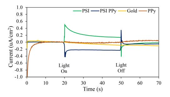
**Figure S6** | *Photoresponse for PSI, PSI-PPy, PPy, and bare gold in 20:1 AscH:DCPIP mediator.*
