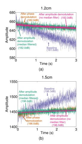
Fig. 5. Amplitude through slow-time is shown for two example depths. For each depth, amplitude is shown for the raw RF data (purple), phase demodulated RF data (orange), and phase & amplitude demodulated RF data with (teal) and without (pink) median filtering. Individual power estimates in dB for each line are shown next to corresponding labels.
