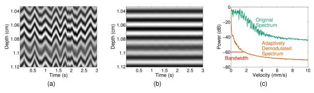
Fig. 2. (a) Example M-mode data before adaptive demodulation. (b) Example M-mode data after adaptive demodulation. (c) The average spectrum through slow-time before adaptive demodulation is shown in teal. The average spectrum through slow-time after adaptive demodulation is shown in orange. Example half-width bandwidth estimate at -60dB is shown in red.
