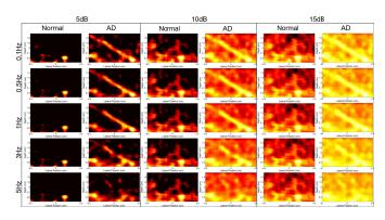
Fig. 12. Power Doppler images of the 1mm/s peak velocity simulation with and without adaptive demodulation (AD) (left and right in each column, respectively) are shown for dynamic ranges between 5 and 15dB (columns) with filter cutoffs between 0.1Hz and 5Hz (rows).
