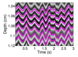
Fig. 1. Displacement profiles in pink superimposed on top of corresponding RF lines through slow-time are shown for several depths.
