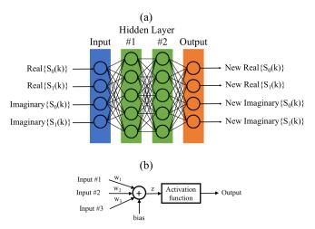
Fig. 3. (a) Example feed-forward multi-layer fully connected network setup for a two element array. The inputs to the network were separated into real and imaginary components. Information only moves from left to right. (b) Diagram for a single neuron.
