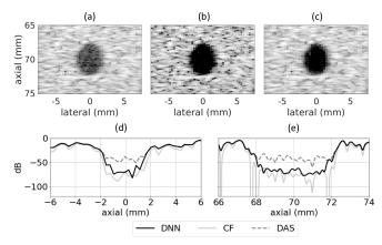
Fig. 9. Simulated 5 mm diameter anechoic cyst at 70 mm depth using (a) DAS, (b) CF, and (c) DNNs. (d) Lateral and (e) axial profiles through the center of the cyst. White Gaussian noise was added such that the channel SNR was 20 dB. Images are shown with a 60 dB dynamic range.
