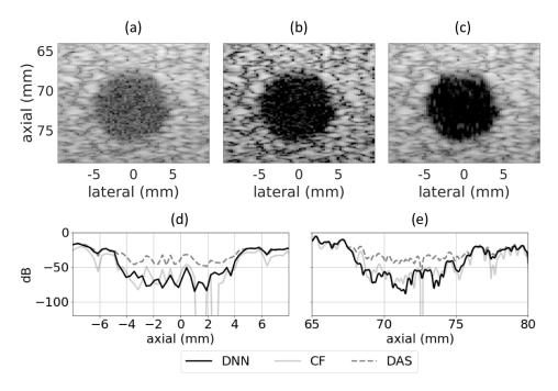
Fig. 10. Phantom 5 mm diameter anechoic cyst at 70 mm depth using (a) DAS, (b) CF, and (c) DNNs. (d) Lateral and (e) axial profiles through the center of the cyst. Images are shown with a 60 dB dynamic range.
