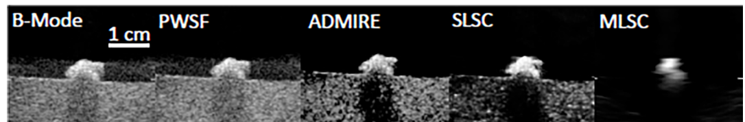
Fig 3. B-mode, PWSF, SLSC, MLSC, and ADMIRE images of a 10mm stone at 8cm depth. Note the posterior shadow appears below each of the stones.
